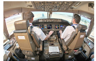
The two-crew glass cockpit has fly-by-wire controls
