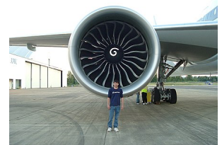
The more powerful GE90 engines of later variants has a 128 in (330 cm) diameter fan up from 123 in (310 cm) in earlier variants, and curved blades instead of straight ones
